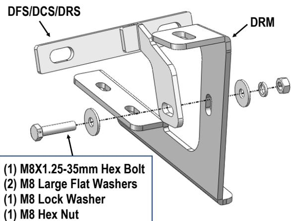
(Fig 8) Driver Rear Mounting Bracket Assembly
