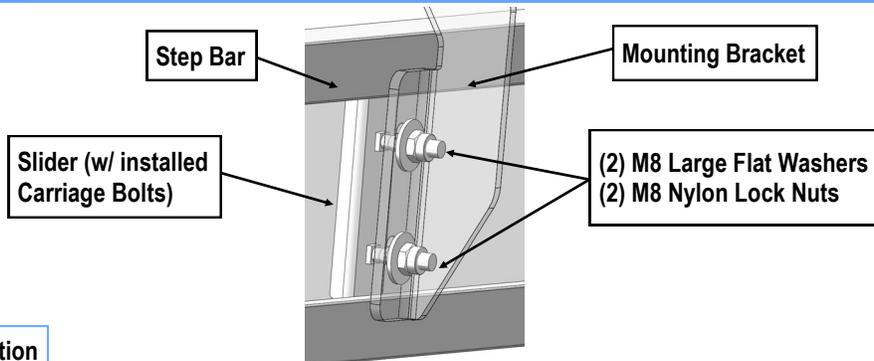
(Fig 14) Step Bar Installation
