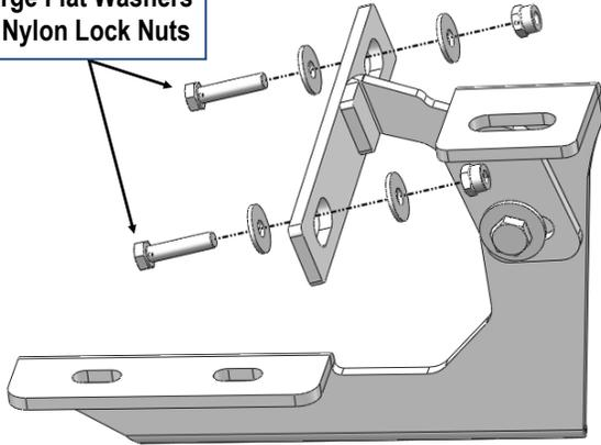
(Fig 9) Driver Front Support Bracket Installation
