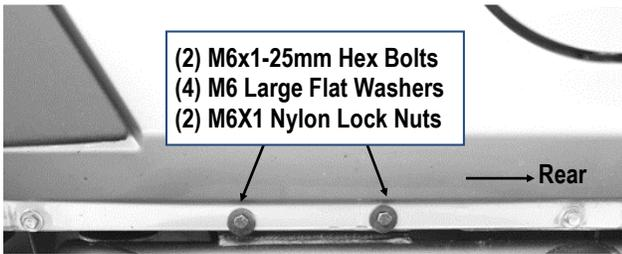
(Fig 10) Driver Front Support Bracket Installed
