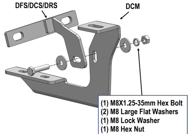
(Fig 7) Driver Center Mounting Bracket Assembly
