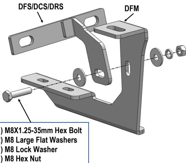
(Fig 6) Driver Front Mounting Bracket Assembly
