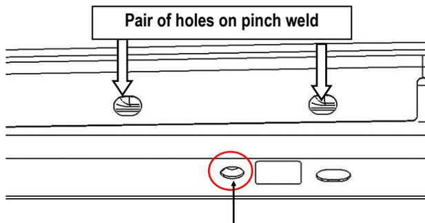
(Fig 2) Line up Nut Plate with hole in between the (2) holes on the pinch weld
