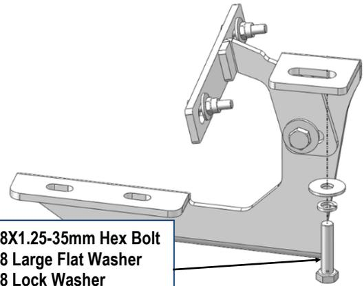
(Fig 11) Driver Front Mounting Bracket Installed
