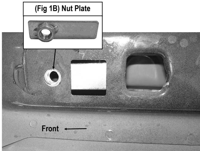
(Fig 1A) Driver Side Front Mounting Location
