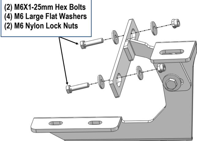
(Fig 8) Driver Front Support Bracket Installation
