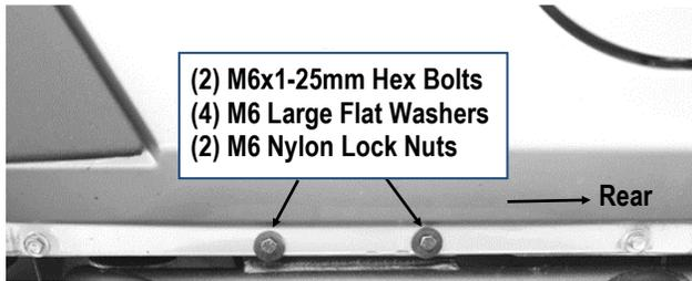
(Fig 9) Driver Front Support Bracket Installed
