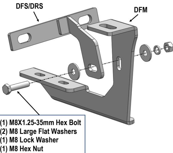
(Fig 6) Driver Front Mounting Bracket Assembly
