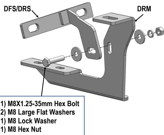
(Fig 7) Driver Rear Mounting Bracket Assembly
