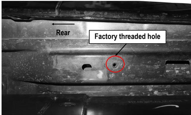
(Fig 5) Driver Side Rear Mounting Location
