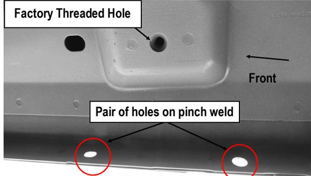
(Fig 4) Passenger Side Rear Mounting Location
