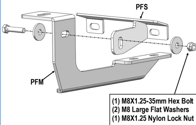
(Fig 1) Passenger Front Mounting Bracket Assembly
