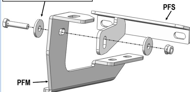
(Fig 5) Passenger Rear Mounting Brackets Assembly
