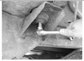
(Fig 1) Remove Factory Body Mount Bolt
