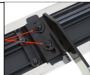
(Fig 10) Step Bar Installed on Bracket Installed (Example)
