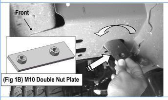
(Fig 1A) M10 Double Nut Plate Installation Driver Front Mounting Bracket (DFM) Location
