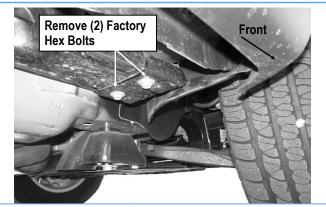
(Fig 8) Passenger Side Front Mounting Location
