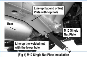
(Fig 4) M10 Single Nut Plate Installation (On the Driver Side Rear Mounting Location)
