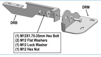
(Fig 3) Driver Rear Mounting Bracket Assembly
