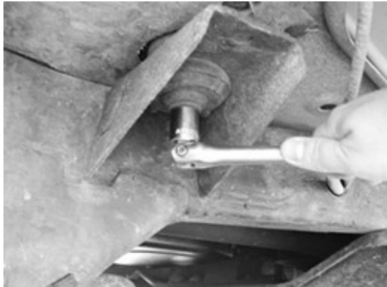
(Fig 1) Remove Factory Body Mount Bolt
