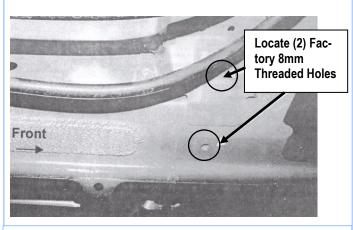
(Fig 4) Driver Side Center Mounting Location
