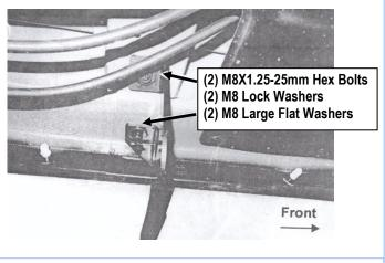
(Fig 5) Driver Center Mounting Bracket Installation
