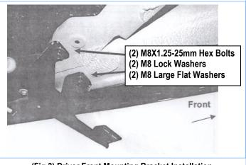
(Fig 3) Driver Front Mounting Bracket Installation
