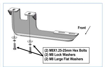
(Fig 2) Driver Front Mounting Bracket Installation
