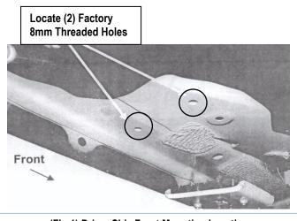
(Fig 1) Driver Side Front Mounting Location
