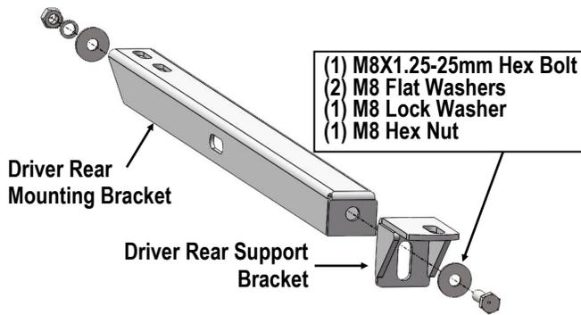
(Fig 9) Driver Side Rear Brackets Assembly
