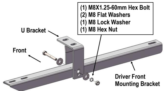
(Fig 8) Driver Front Mounting Bracket Installed
