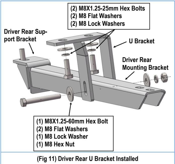
(Fig 11) Driver Rear U Bracket Installed
