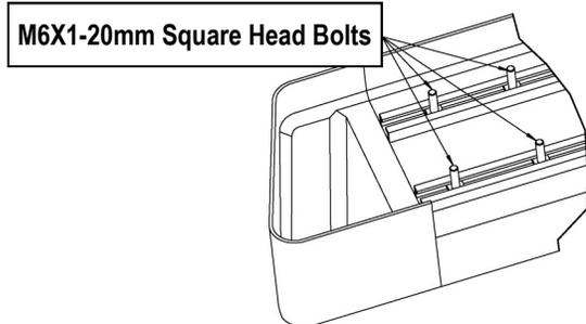
(Fig 12) Slip M6X1-20mm Square Head Bolts Into The Bottom Channels
