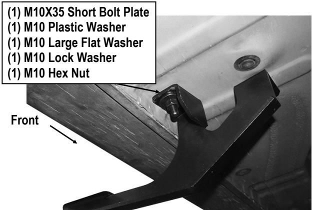
(Fig 7) Driver Side Center Mounting Bracket Installed
