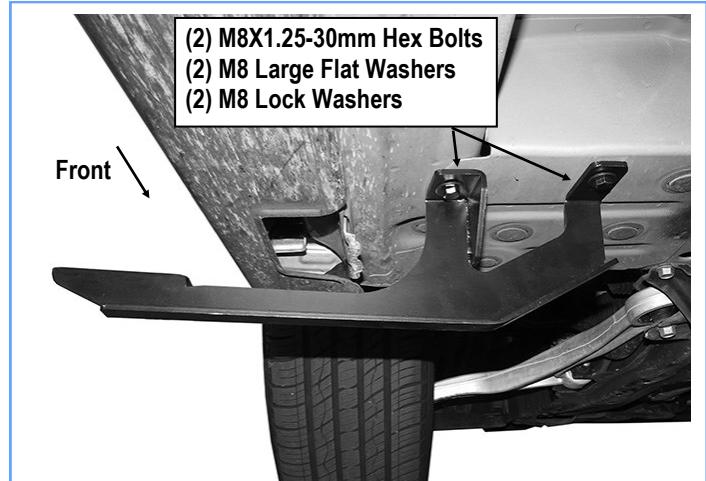
(Fig 3) Driver Side Front Mounting Bracket Installed
