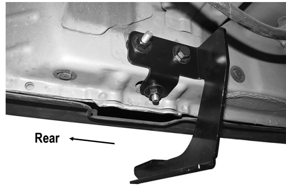
(Fig 11) Driver Side Rear Mounting Bracket Installed
