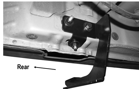
(Fig 11) Driver Side Rear Mounting Bracket Installation
