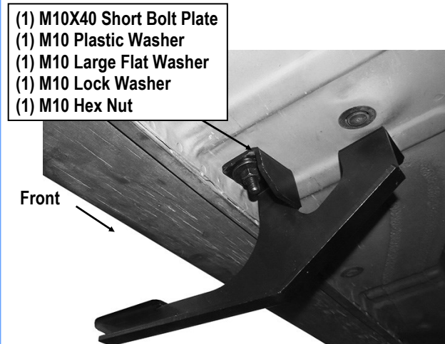
(Fig 7) Driver Side Center Mounting Bracket Installation
