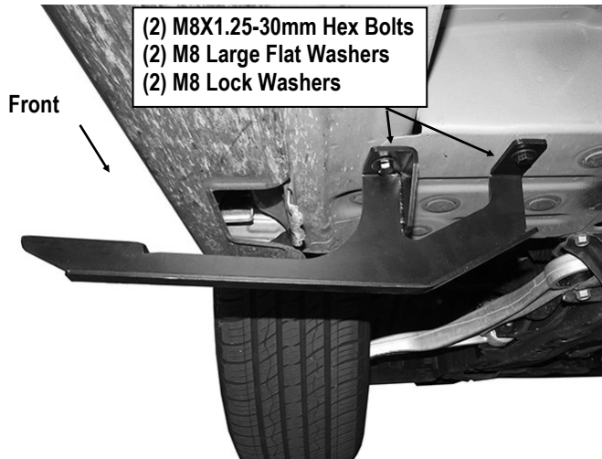
(Fig 3) Driver Side Front Mounting Bracket Installation
