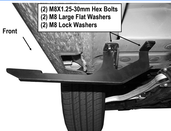
(Fig 3) Driver Side Front Mounting Bracket Installed
