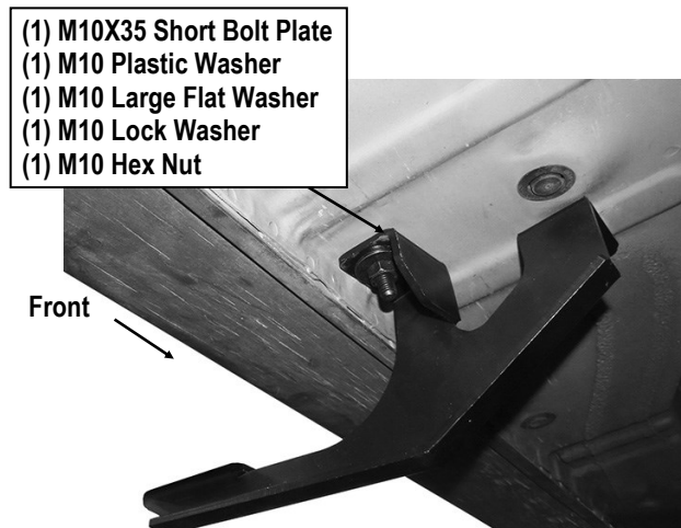
(Fig 7) Driver Side Center Mounting Bracket Installation
