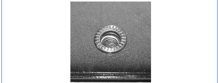
(Fig 11) Tighten Hex Bolt To Collapse And Lock Threaded Insert Into Factory Hole
