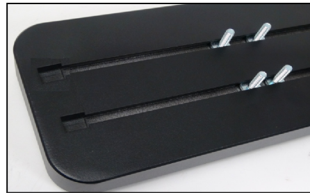
(Fig 12) Slip (2) M6X1-20mm Square Head Bolts Into Each Bottom Channel
