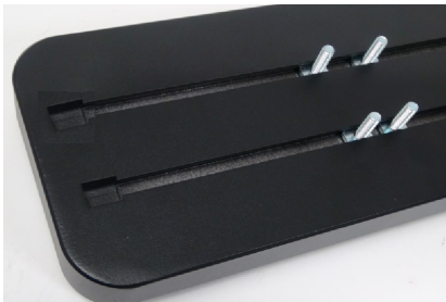
(Fig 14) Slip M6X1-20mm Square Head Bolts Into The Bottom Channels
