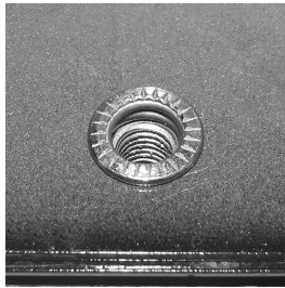
(Fig 11) Tighten Hex Bolt To Collapse And Lock Threaded Insert Into Factory Hole
