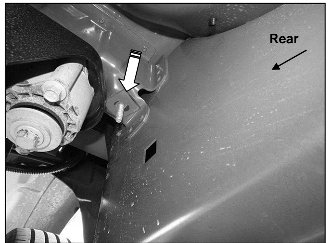
(Fig 10) Insert T-Bolt and folded Washer into oval hole. Thread second Plastic Washer onto T-Bolt
