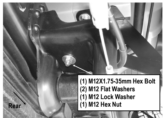
(Fig 19) Driver Side Rear Bracket Completely Installed (2011-2016)
