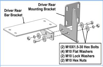
(Fig 10) Driver Rear Brackets Assembly
