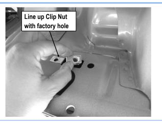
(Fig 8) Driver Side Center Mounting Location (Example)
