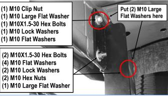
(Fig 6) Driver Side Front Mounting Bracket Installed
