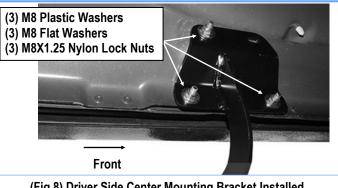
(Fig 8) Driver Side Center Mounting Bracket Installed
