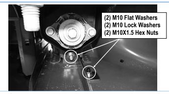
(Fig 15) The Assembled Driver Rear Mounting Bracket Installed
