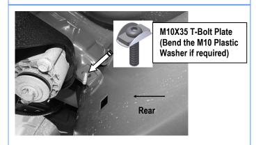
(Fig 11) Insert M10X35 T-Bolt W/ Plastic Washer into oval hole. Thread another M10 Plastic Washer onto T-Bolt
