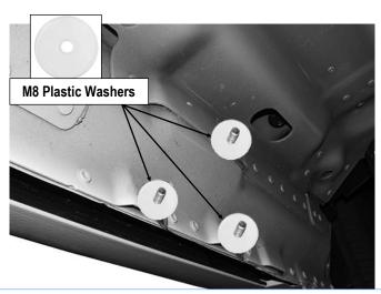
(Fig 5) Driver Side Front Mounting Location
