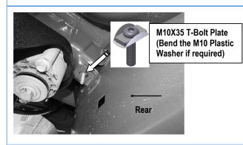
(Fig 11) Insert M10X35 T-Bolt W/ Plastic Washer into oval hole.
