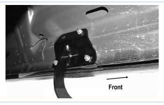
(Fig 7) Driver Front Mounting Bracket Installed
