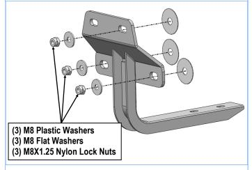
(Fig 6) Driver Front Mounting Bracket Installation
