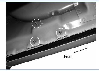
(Fig 4) Driver Side Front Mounting Location
