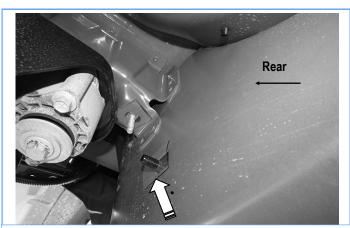
(Fig 13) Insert M10X40 Bolt Plate W/Plastic Washer into square hole. Thread another Plastic Washer onto Bolt Plate
