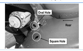
(Fig 9) Driver Side Rear Mounting Location
