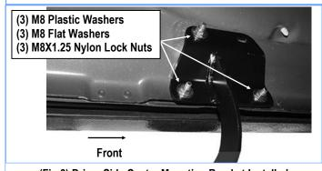
(Fig 8) Driver Side Center Mounting Bracket Installed
