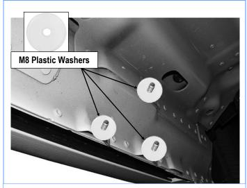
(Fig 5) Driver Side Front Mounting Location
