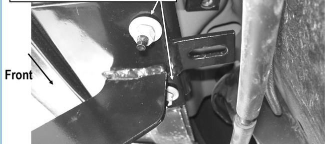
**(Fig 2) Driver Front Mounting Bracket Installation**
