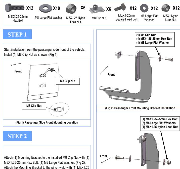
Attach the Mounting Bracket to the pinch weld with (1) M8X1.25 -25mm Hex Bolt, (2) M8 Large Flat Washers and (1) M8X1.25 Nylon Lock Nut, **(Fig 3).** Do not fully tighten hardware at this time.
