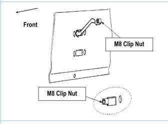
(Fig 1) Passenger Side Front Mounting Location
