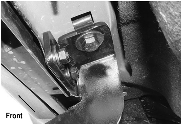
(Fig 4) Passenger Front Mounting Bracket Installation
