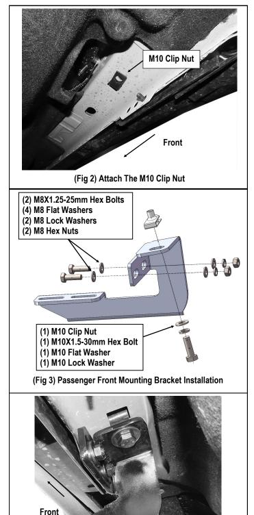
(Fig 4) Passenger Front Mounting Bracket Installation
