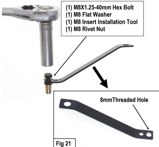
(Fig 20) Assemble Insert Tool As Pictured
