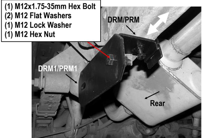
(Fig 6) Passenger Rear Mounting Bracket 1 Installation
