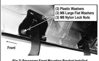
(Fig 3) Passenger Front Mounting Bracket Installed
