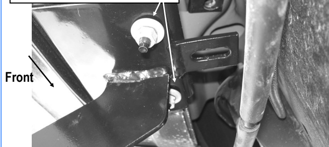
(Fig 2) Driver Front Mounting Bracket Installation
