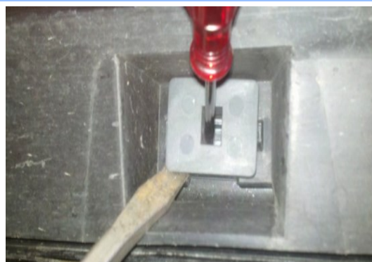
(Fig 2) Remove The (2) Forward Most Retainers
