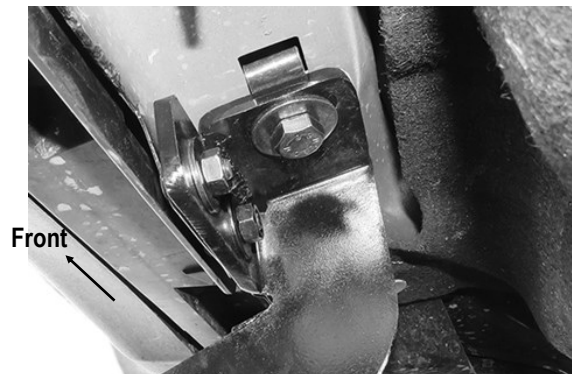
(Fig 4) Passenger Front Mounting Bracket Installation
