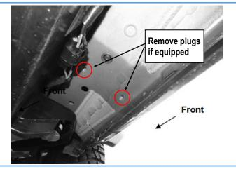
(Fig 1) Passenger Side Front Mounting Location
