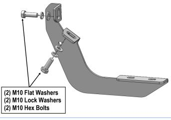
(Fig 6) Passenger Rear Mounting Bracket Installation
