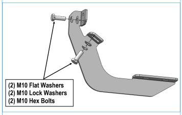
(Fig 4) Passenger Center Mounting Bracket Installation
