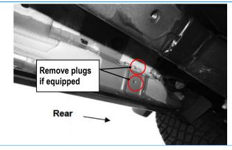
(Fig 5) Passenger Side Rear Mounting Location
