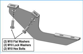
(Fig 2) Passenger Front Mounting Bracket Installation
