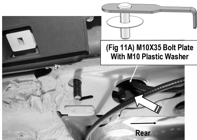
(Fig 11) Insert 10mm Bolt Plate Installation (On Driver Side Rear Mounting Location)
