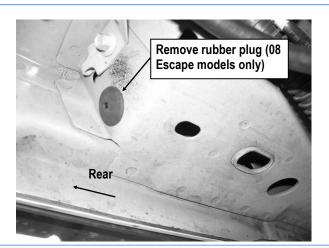
(Fig 8) Driver Side Rear Mounting Location
