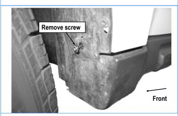
(Fig 1) Remove Screw from the front fender
