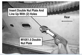
(Fig 9) M10X1.5 Double Nut Plate Installation
