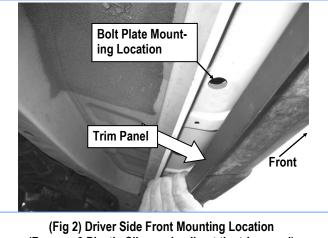
(Remove 3 Plastic Clips and pull out the trim panel)
