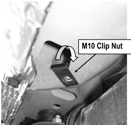
(Fig 1) M10 Clip Nut Installed
