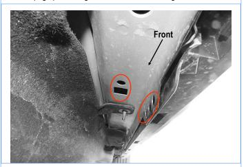
(Fig 6) Passenger Side Rear Mounting Location
