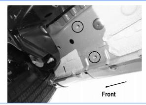
(Fig 1) Passenger Front Mounting Bracket Location
