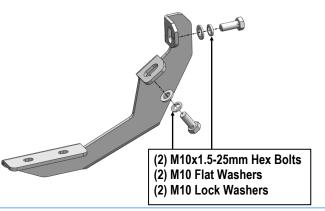
(Fig 5) Passenger Center/Rear Mounting Bracket Installation
