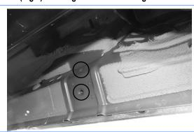
(Fig 4) Passenger Rear Mounting Location
