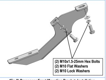
(Fig 2) Passenger Front Mounting Bracket Installation
