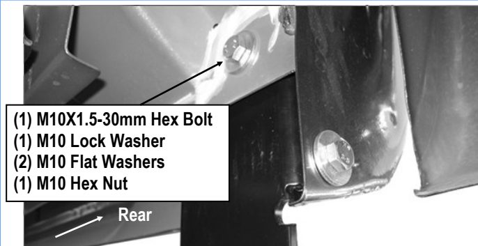
(Fig 4) Passenger Rear Mounting Bracket (PRM) Installation
