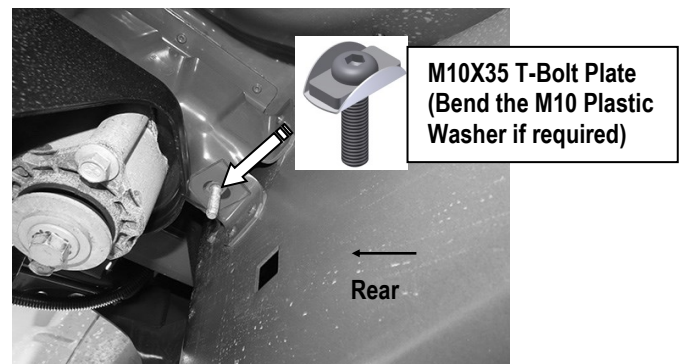
(Fig 8) Insert M10X35 T-Bolt W/ Plastic Washer into oval hole. Thread another M10 Plastic Washer onto T-Bolt
