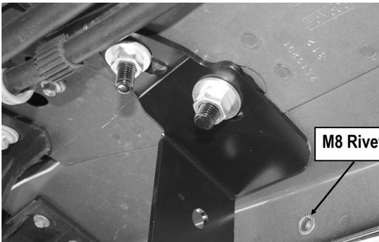
(Fig 15) M8 Rivet Nut Installed on Pinch Weld (Driver Rear Support Bracket Location)
