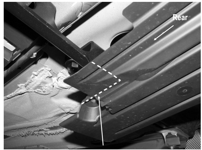
(Fig 13) Hold Plastic Cover back to the Position, Mark the Trimming Area
