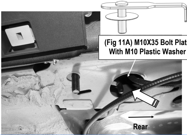
(Fig 11) Insert 10mm Bolt Plate Installation (On Driver Side Rear Mounting Location)
