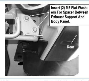
(Fig 11) Passenger Rear Mounting Bracket (09-010 models: Install Mounting Bracket Between Exhaust Support And Body Panel)
