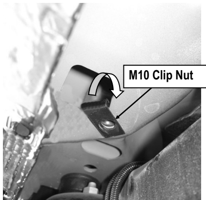
(Fig 1) M10 Clip Nut Installed
