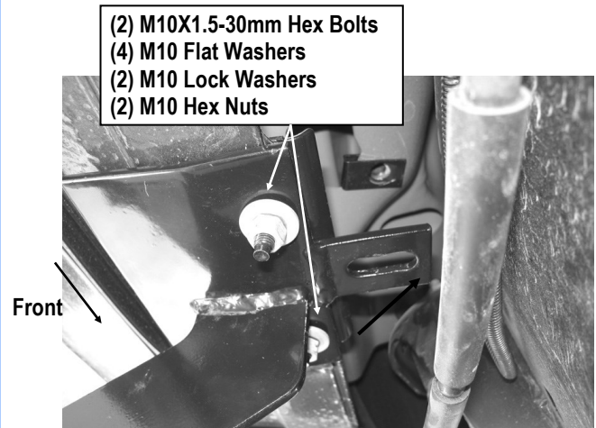
(Fig 3) Driver Front Mounting Bracket Installation
