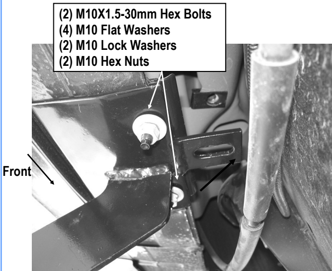
(Fig 3) Driver Front Mounting Bracket Installation
