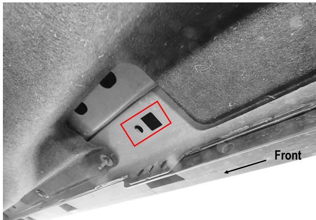
(Fig 5) Passenger Side Center Mounting Location
