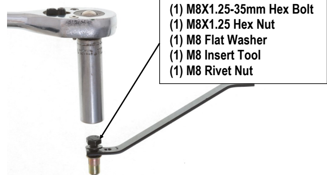
(Fig 20) M8 Insert Tool Assembly
