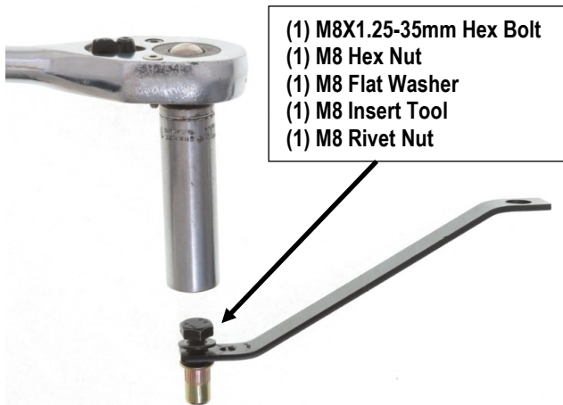
(Fig 17) M8 Insert Tool Assembly
