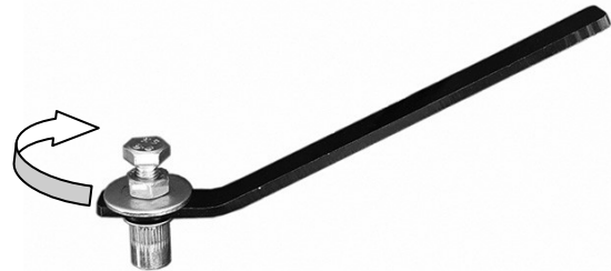
(Fig 19) M8 Insert Tool Assembly
