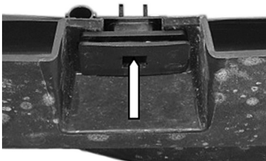
(Fig 1) Insert Flat Screwdriver Into Square Opening to Release the Plastic Clip
