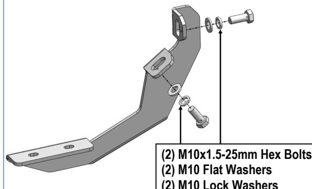
(Fig 5) Passenger Center/Rear Mounting Bracket Installation
